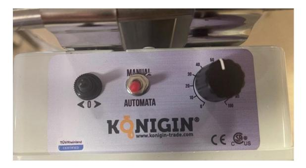
**Manual Mode:** Set your speed using the dial on the right hand. The extractor will gradually increase velocity until the desired speed is reached. This mode is ideal for tangential or radial extractors.
